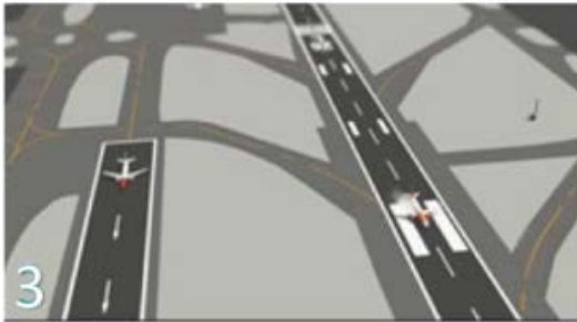
3 As the aircraft approaching the southern runway touches down, the second aircraft on the northern runway is given take-off clearance.
