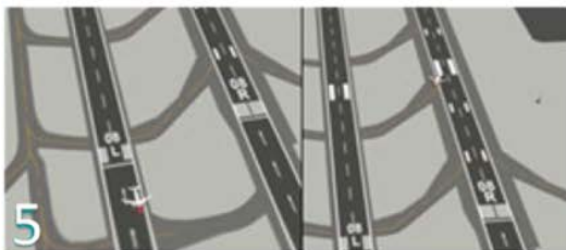
5 The departure on the northern runway lifts-off and starts to climb away and the arrival aircraft vacates the southern runway using one of the exit taxiways.
