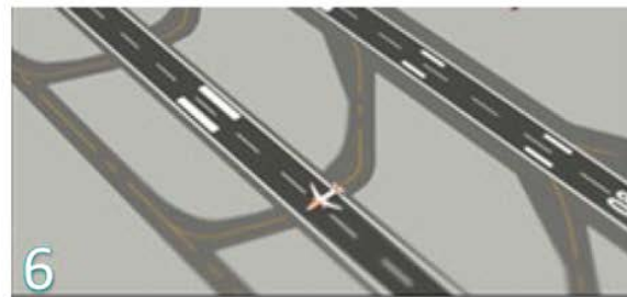
6 The arrival aircraft is instructed to cross the northern runway behind the departure aircraft that has climbed away.
